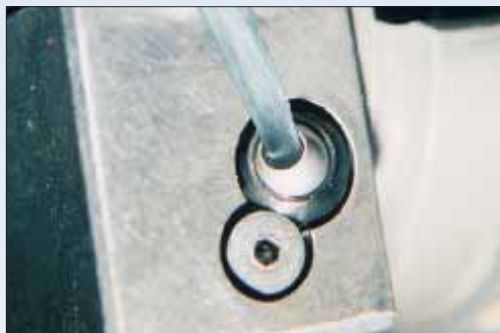
Black Eye installed on quick change turning tool.
