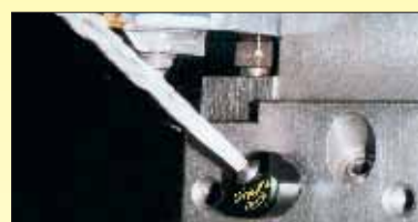
TurretJet shown installed in lathe turret.
