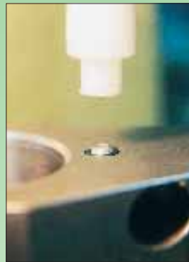
3 Press in JiffyJet until body is flush.
