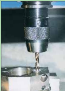
1 Drill coolant passage, leaving reaming allowance.
