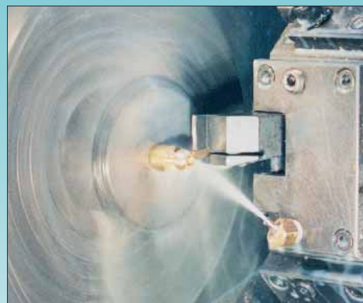
PressureMax nozzle shown in use on CNC turning center. High velocity coolant stream prolongs tool life and aids chip control.
